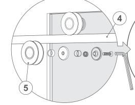
Hang the shower door on the guide rail using the previously installed rollers. If the walls are not completely vertical or an adjustment must be made to make the door fit properly, an adjustment can be made on the rollers. Simply loosen the hex screw with the provided Allen key on each roller and make the necessary adjustment.
