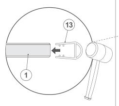
You should now have the stationary glass attached to the guide rail. Place the seal strip (13) on the stationary glass and proceed by installing the wall mount brackets (3), wall brackets (8) and threshold holder (10) on the stationary glass as shown on the figure:
